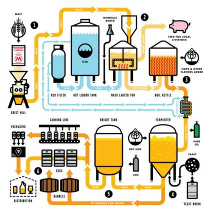
Figure 1: Flow diagram of the brewing process (Trosset, 2018).
