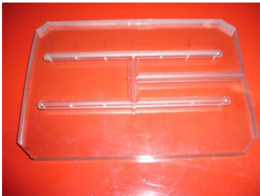
Figure 11: Preliminary Design - Irrigation Trough Lid
