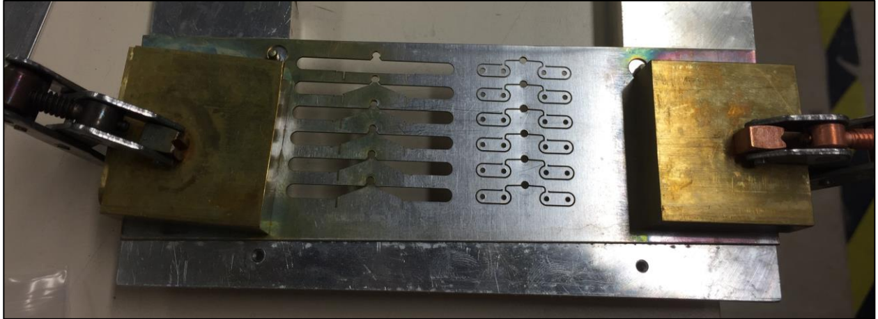
Figure 36: Sheet of metal from which the blade and linkages were cut
