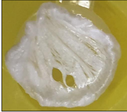
Figure 50: Bovine tendon lacking uniformity and integrity
