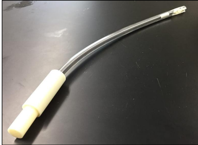
Figure 23: Fully assembled prototype with reverse scissor mechanism, flexible sheathing, and push button mechanism
