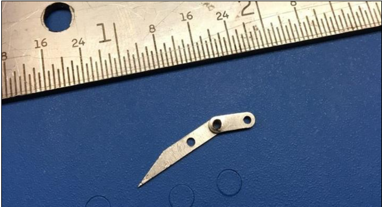
Figure 39: Blade and linkage assembled with peened miniature stainless steel tubing
