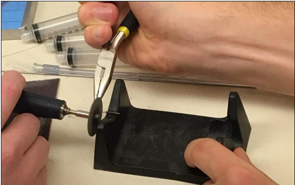
Figure 37: Cutting the miniature stainless steel tubing to size using a rotary tool with a cut-off wheel attachment
