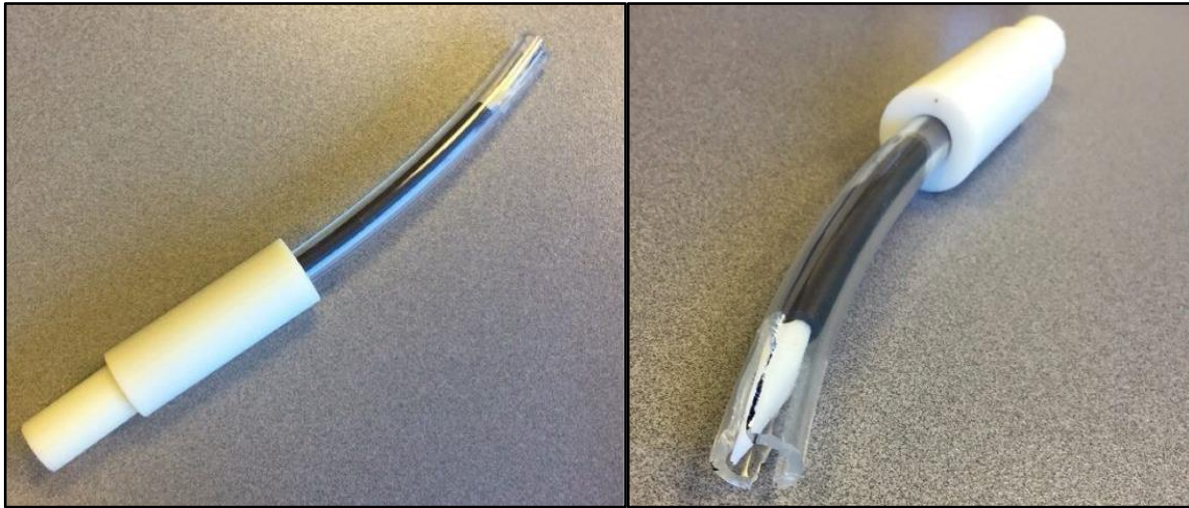
Figure 13: Proof of concept of Interchangeable Blade design at 10X scale with 3D printed push button mechanism and blade, an internal spring, polyurethane outer tubing, and silicone inner tubing cut to size
