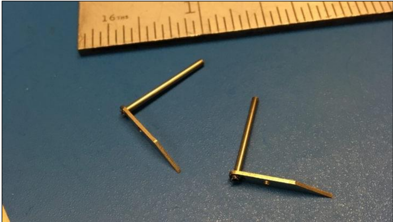
Figure 38: Blades with miniature precision stainless steel tubing laser welded flush to one end
