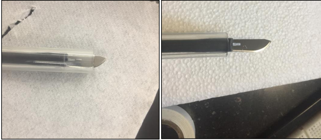
Figure 14: Close up view of the difference in elongation of inner tubing and scalpel blade for the Interchangeable Blade proof of concept
