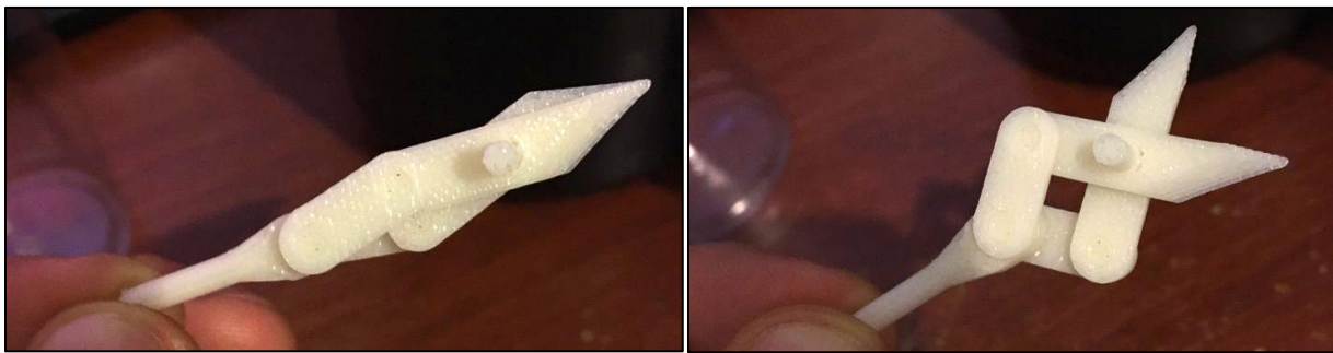
Figure 22: Fully assembled Reverse Scissors mechanism closed (left) and open (right)
