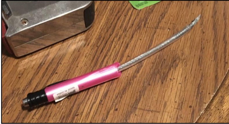
Figure 10: Proof of Concept made with pen mechanism, outer plastic tubing, and inner wire, and a small blade
