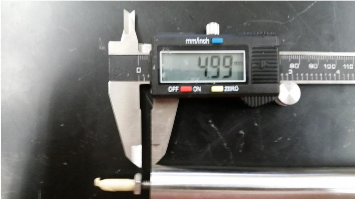
Figure 14: Set up for LVDT validation testing
