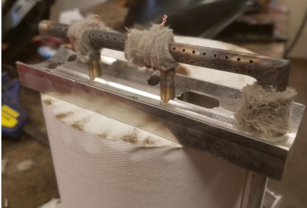
*Figure 13. Burner tube, mounted on the boiler bottom plate*
