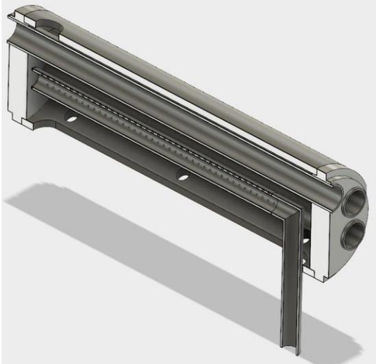
*Figure 8. Sectioned view of the CAD model of the burner pipe, water pipes, endplates, and boiler shell assembly*
