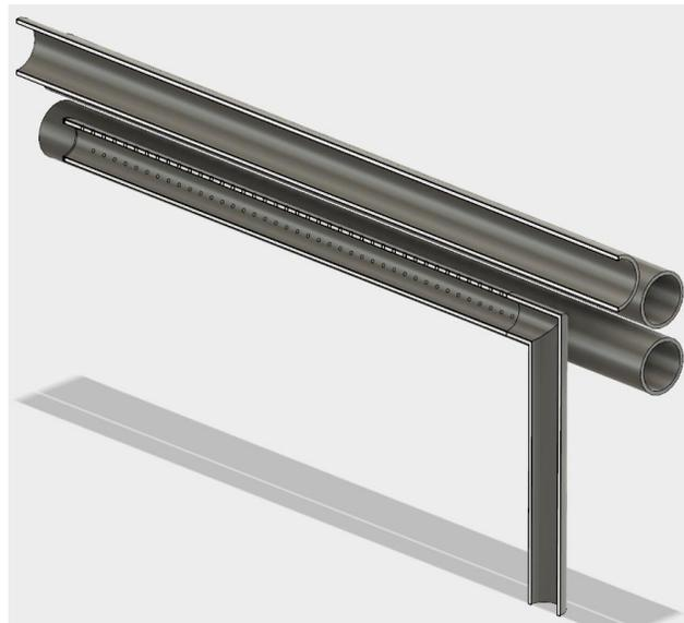
*Figure 6. Sectioned view of CAD model of the burner and water pipes assembly*
