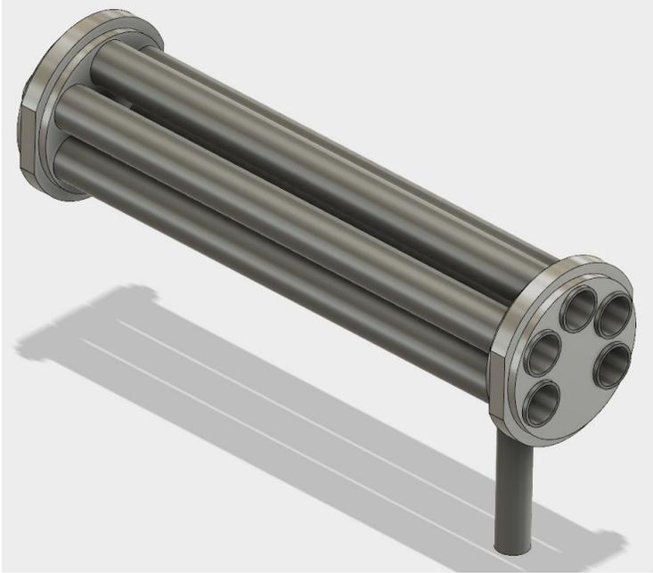
*Figure 7. CAD model of the burner pipe, water pipes, and endplates assembly*
