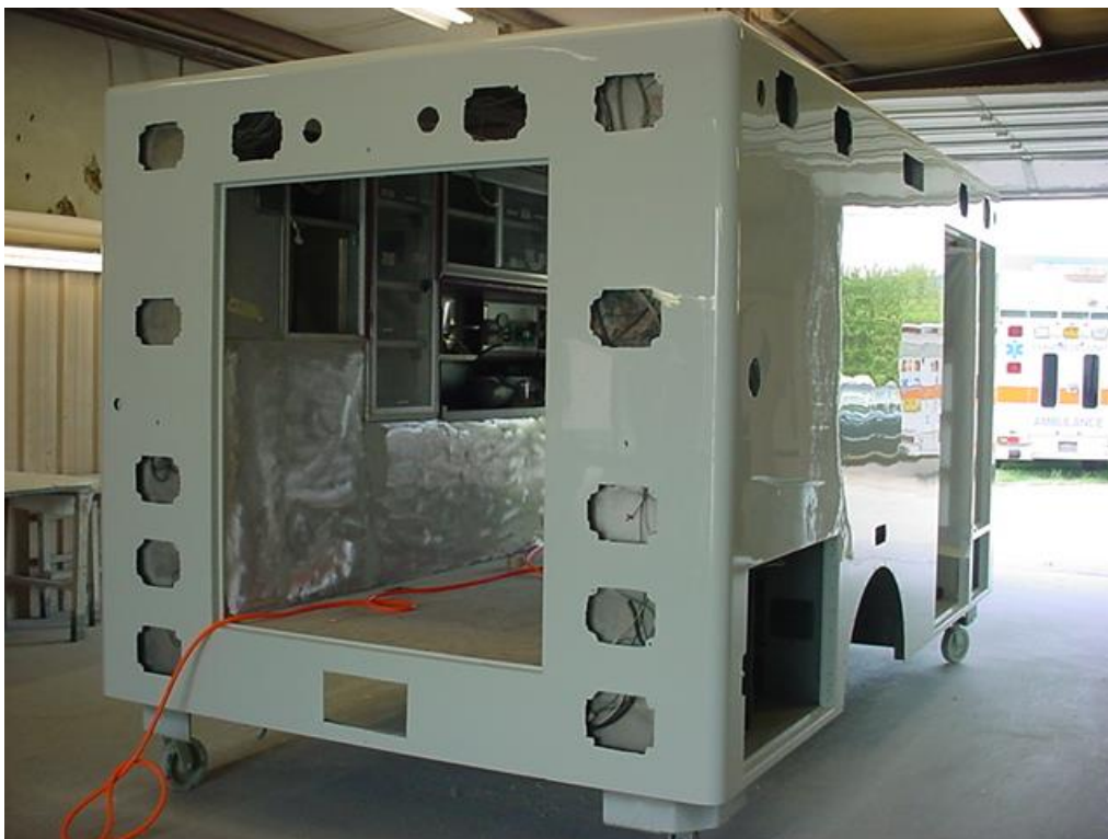
Figure 48: Ambulance rear compartment under construction
