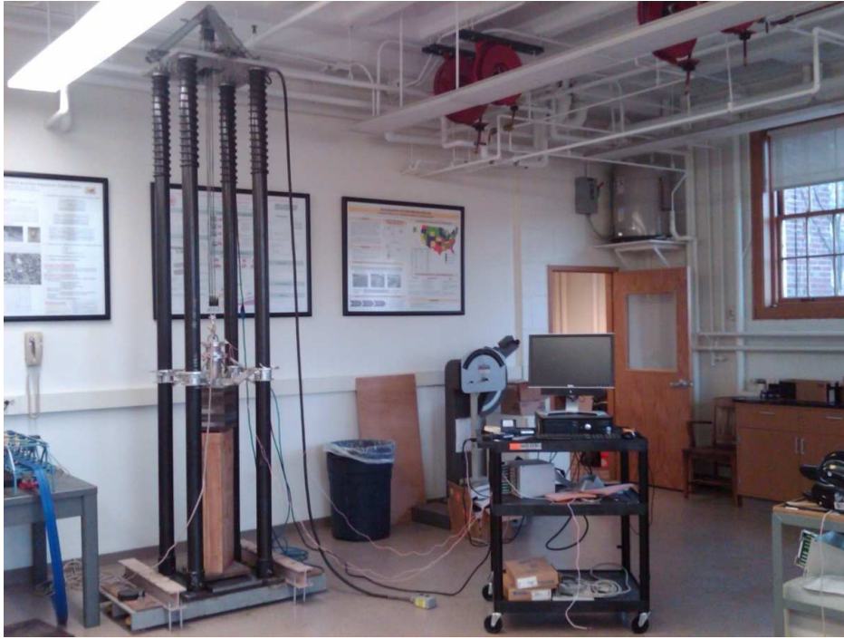
Figure 9: Drop tower workstation for dynamic testing.
