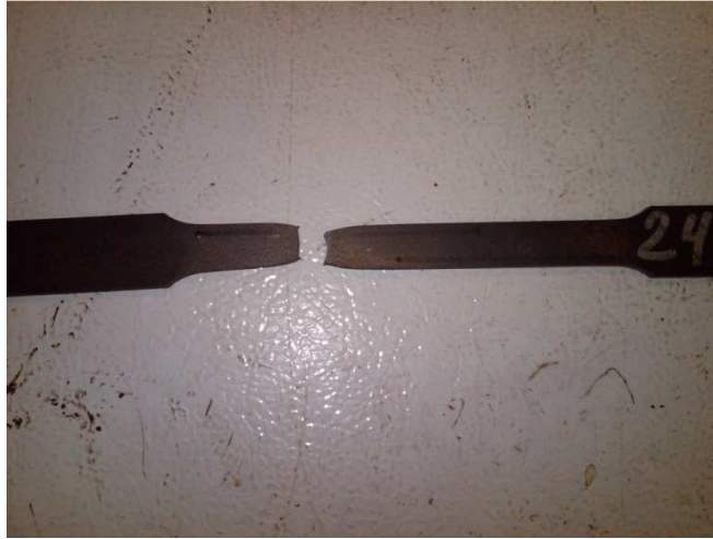
Figure 28: Close-up of tensile bar #3 after testing.
