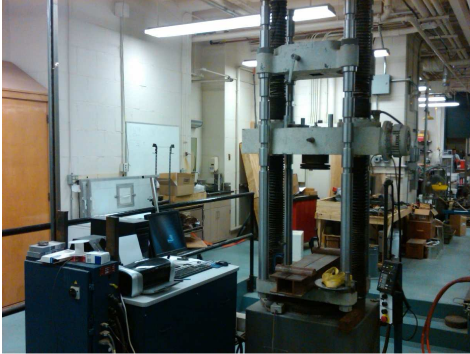
Figure 4: Tinius Olsen Testing Machine workstation for tensile testing and quasi-static testing.
