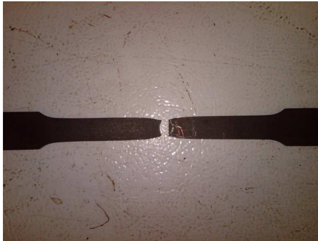
Figure 20: Close-up of tensile bar #1 after testing.
