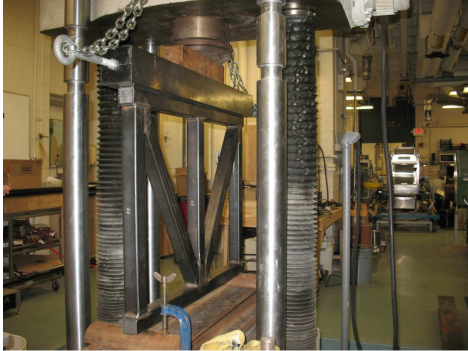
Figure 7: Setup for quasi-static distributed loading on a truss sample.
