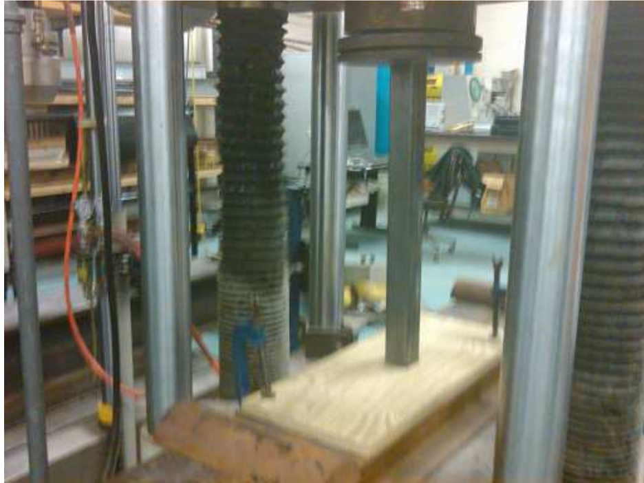
Figure 6: Setup for quasi-static loading on a column sample.
