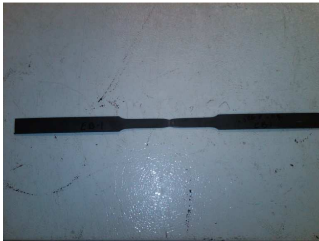
Figure 19: Tensile bar #1 after testing.
