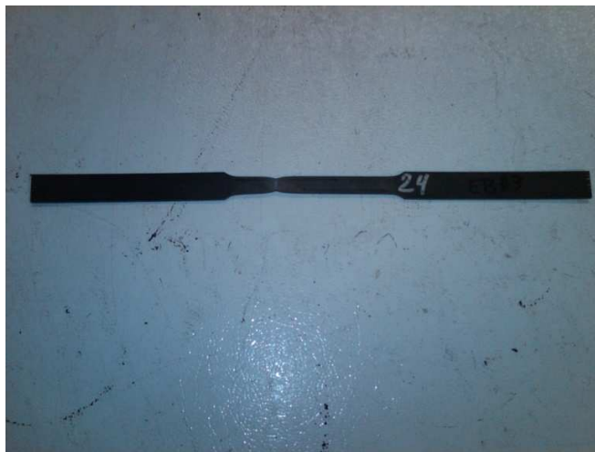
Figure 27: Tensile bar #3 after testing.
