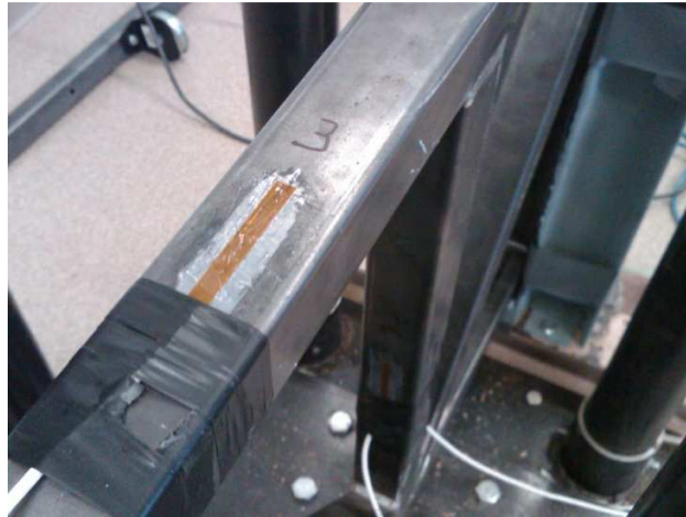
Figure 14: Strain gauge setup on a truss.
