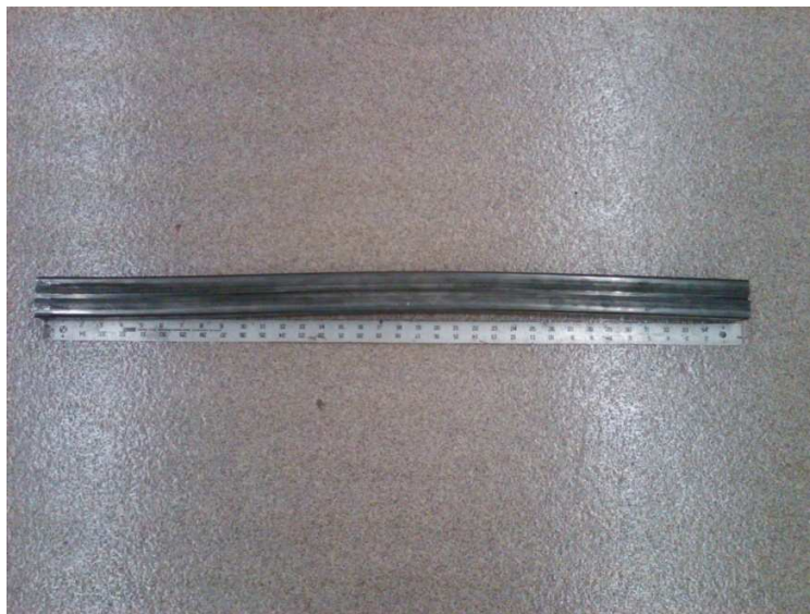
Figure 70: Result from Column (long) dynamic test.
