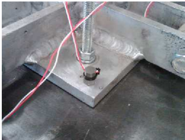
Figure 13: 10,000-g piezoelectric shock accelerometer on impact head
