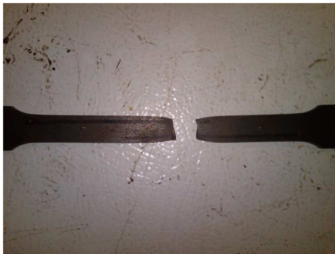
Figure 24: Close-up of tensile bar #2 after testing.
