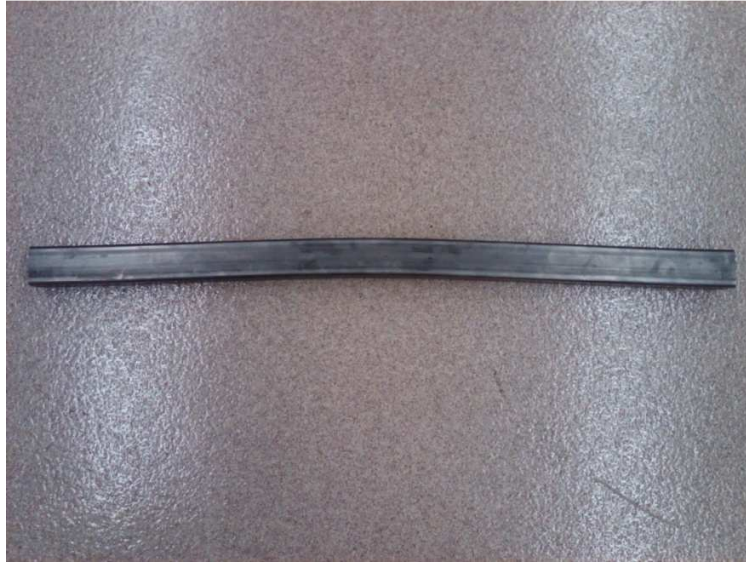
Figure 32: Result from column (long) static test.
