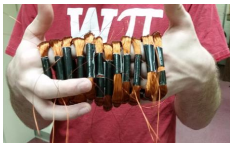
Figure 28: Our twelve coils are shown here. Each of them is three-hundred turns of 28 AWG copper wire.
