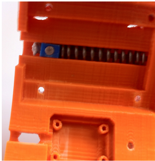
Figure 15: View of SEA mechanism and magnet mount
