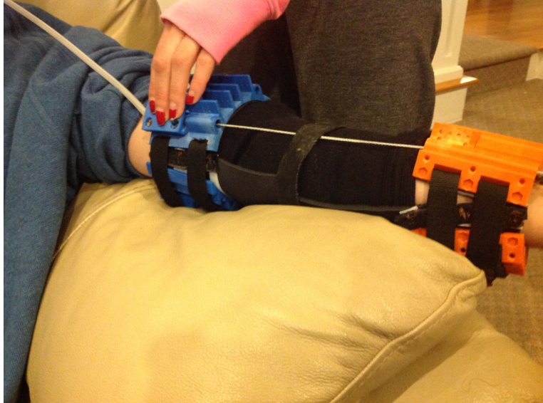
Figure 11: Slippage test for the first prototype of the brace.
