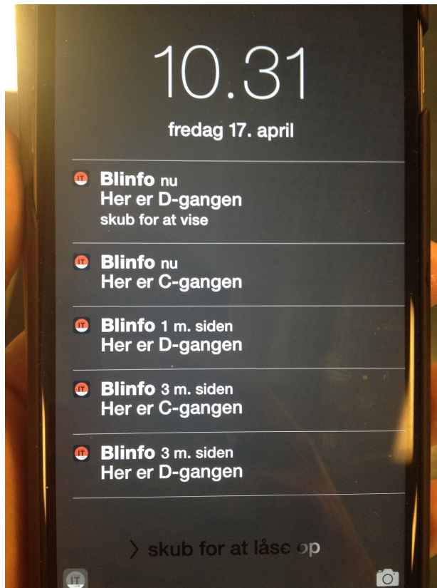
Figure 7: Photo of a smartphone screen with repeated notifications from two iBeacons during testing
