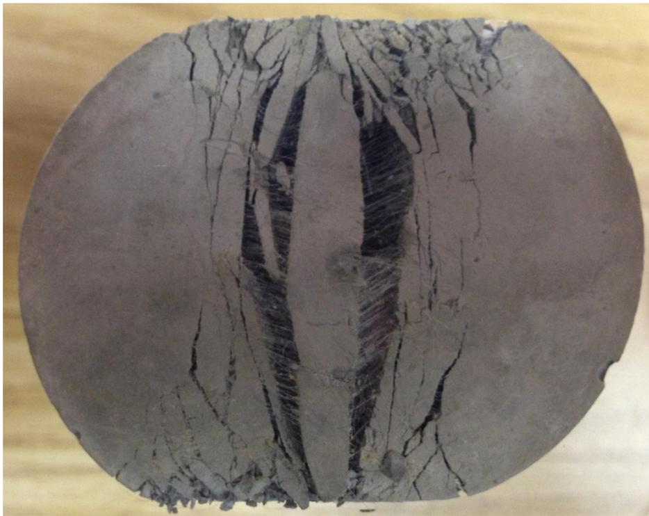
Figure 28: A typical broken fiber-reinforce cement paste sample subjected to split-cylinder test.
