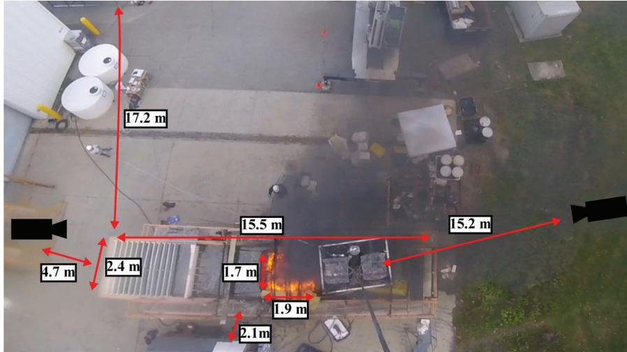
Figure 4.3: Top-down view of wavetank site during a burn, showing linear distances to key locations.
