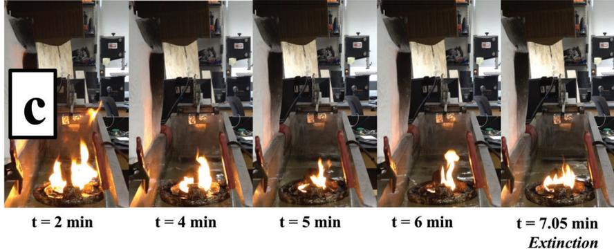
Figure 2.4: Visual timelines for three different wave profiles: (a) no-wave, (b) wave 2, (c) wave 9.
