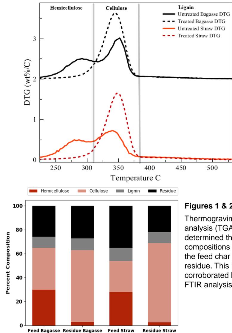
Figures 1 & 2: Thermogravimetric analysis (TGA) determined the compositions of the feed char residue. This is corroborated by FTIR analysis.
