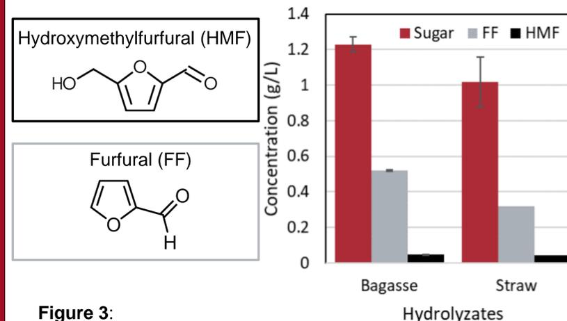
Figure 3: UV-Vis spectroscopy and high-performance liquid chromatography (HPLC) determined sugar and inhibitor concentrations.
