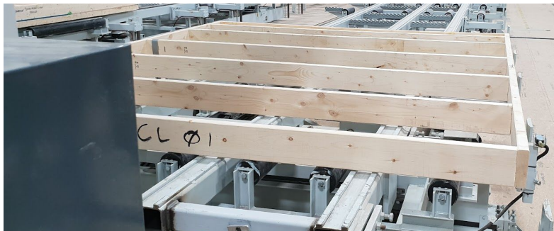
Figure 3. Unity Homes - Open Panel Frame
