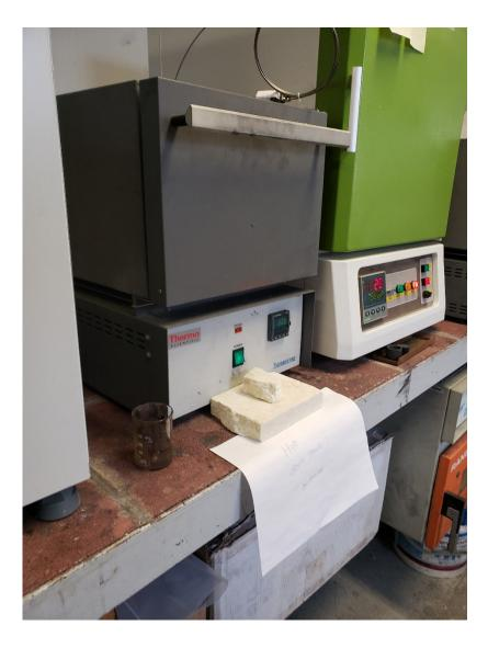
Thermo Scientific Furnace used for Quenching and Annealing
