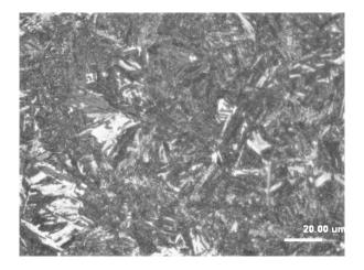
Figure 28: Austempered 30 min 500X under the microscope (Intermediate)
