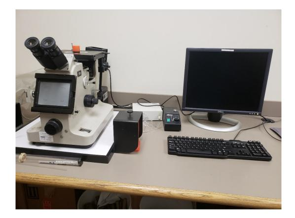
Nikon Microscope used for optical tests
