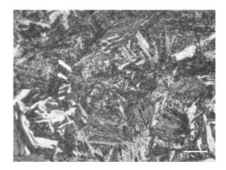
Figure 25: Austempered 5 Min 1000X under the microscope (Center)
