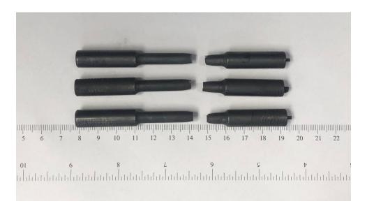
Tensile Testing Bars (30 minutes)
