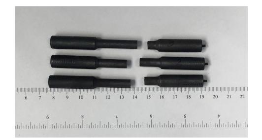
Tensile Testing Bars (5 minutes)
