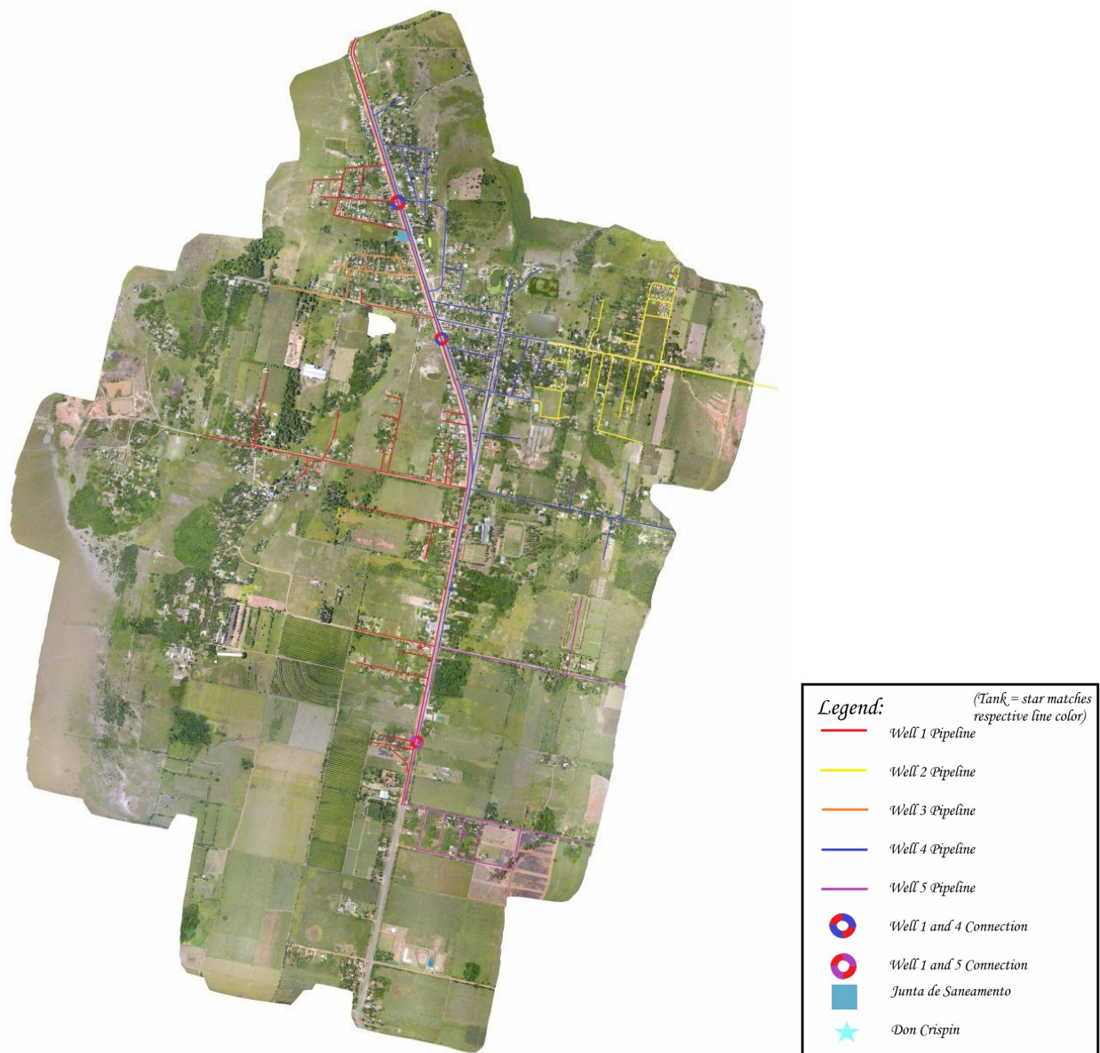
Figure 2: Community Clean Water Access Pipeline Map of the Junta de Saneamiento (Community Clean Water Access, 2018)
