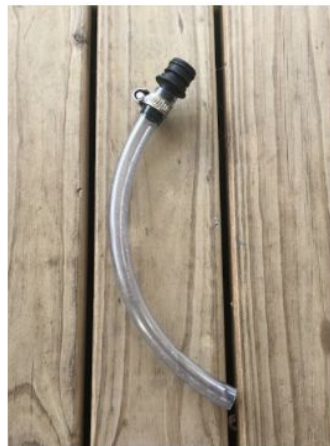
Assembled Pump Outlet Connection
