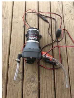
Assembled Pump with inlet and outlet
