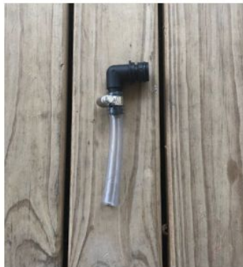
Assembled Pump Inlet Connection
