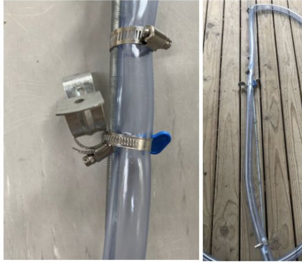
Assembled Inlet Tube
