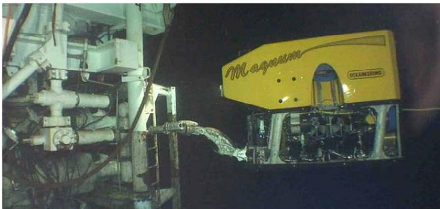
*Figure 3: Partially Autonomous ROV Working on Pipeline*
