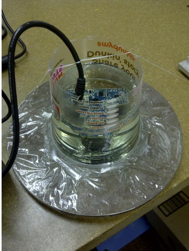
*Figure 53: Epoxy Application to Waterproof Housing*
