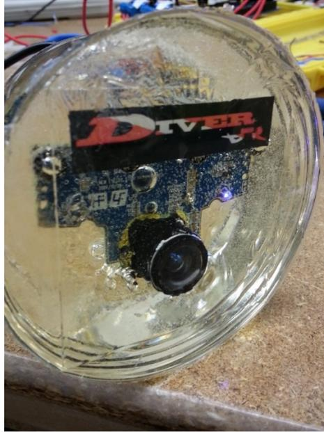
*Figure 54: Camera Housing Completed*
