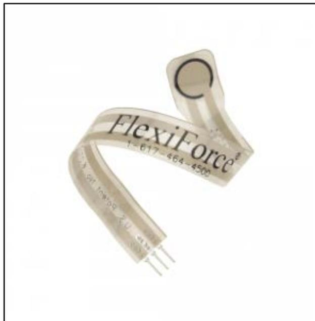
Figure 56: Parallax Pressure Sensor
