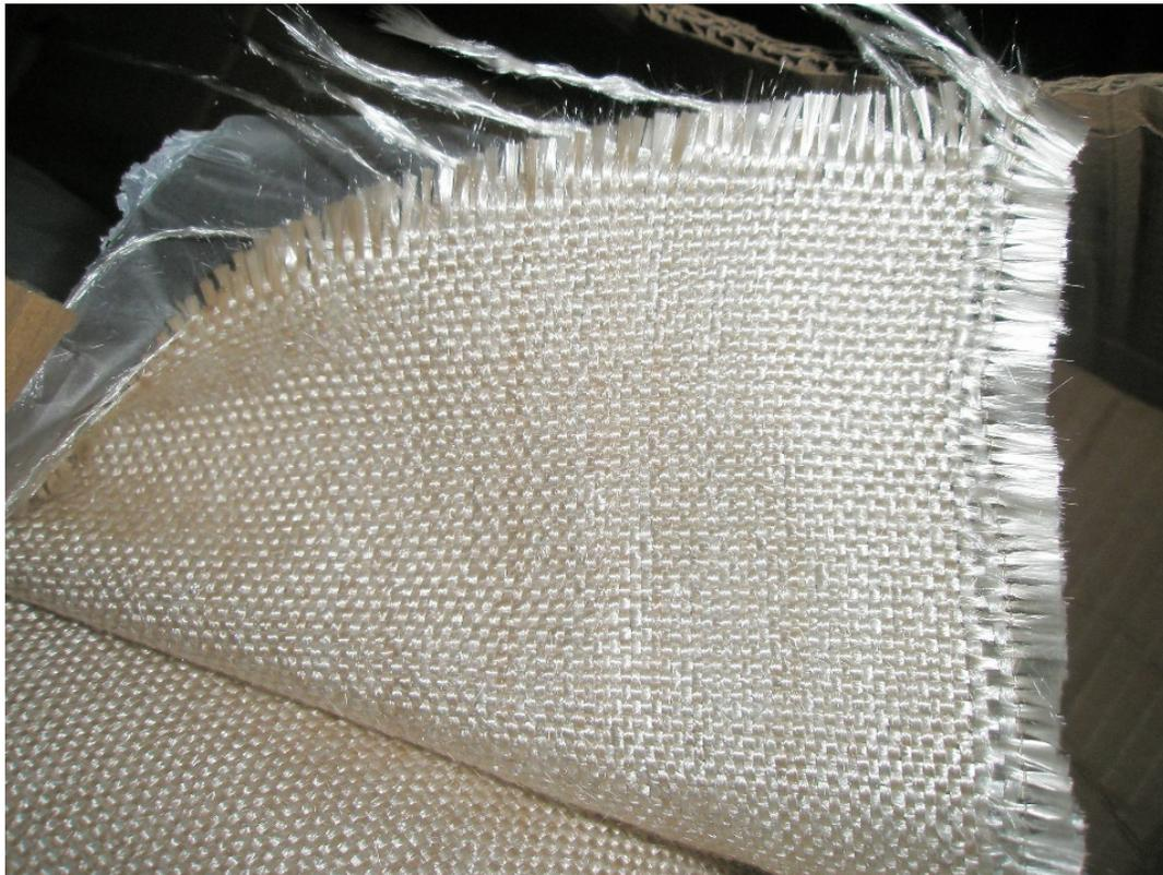
*Figure 25: Fiberglass Mesh*
