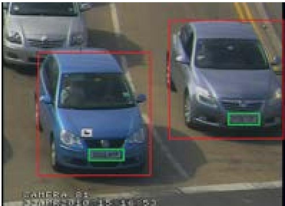
*Figure 9: Detecting license plates for traffic management*
