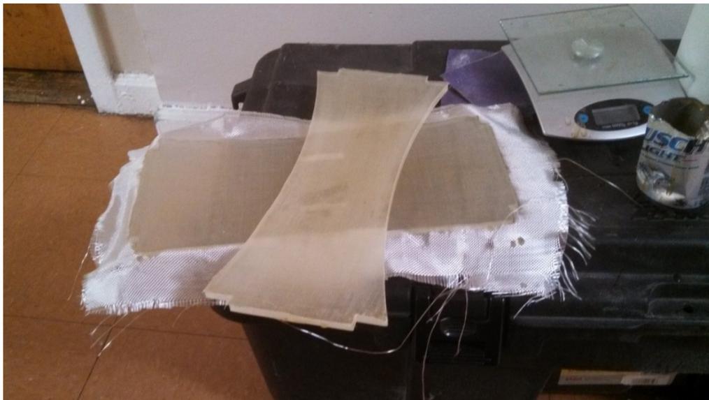
*Figure 28: Fiberglass Reinforcement*
