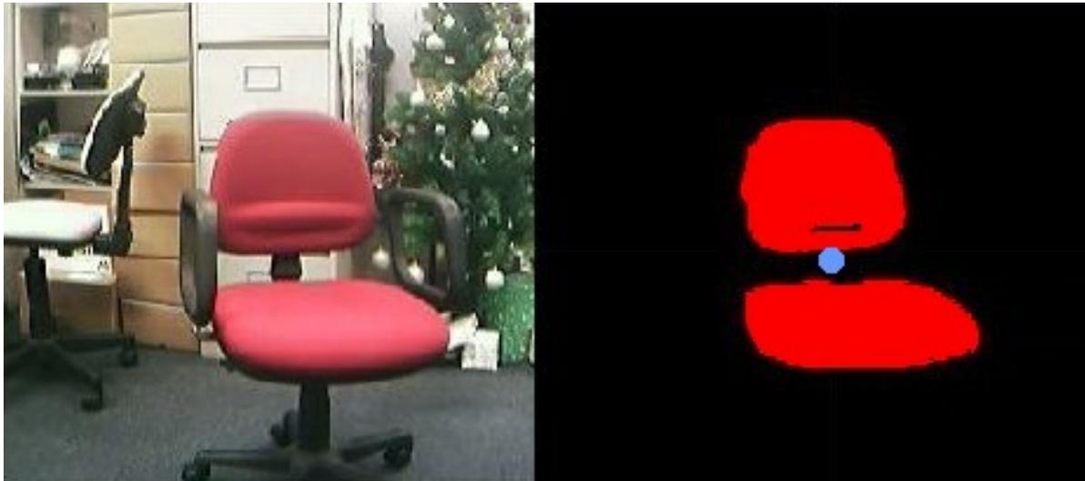
*Figure 10: Detecting a Red Object using Blob Detection*
