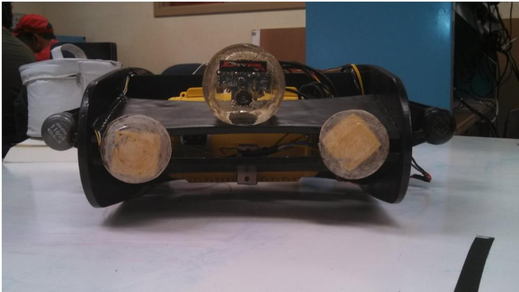
*Figure 49: LED Light Arrays on Front of DIVER ROV*
