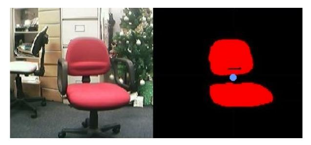
Figure 10: Detecting a Red Object using Blob Detection
