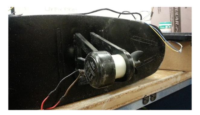
Figure 34: Horizontal Thruster Assembly
