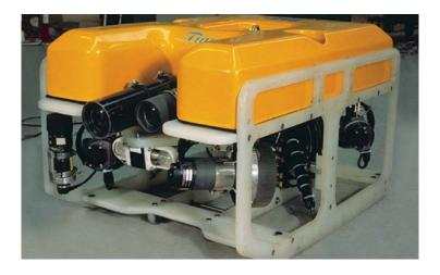
Figure 2: An Observation Class ROV with Lights and Camera
