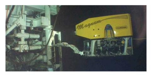
Figure 3: Partially Autonomous ROV Working on Pipeline
