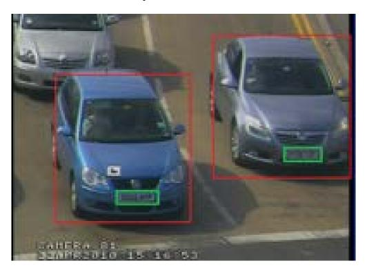
Figure 9: Detecting license plates for traffic management
