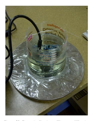
Figure 53: Epoxy Application to Waterproof Housing
