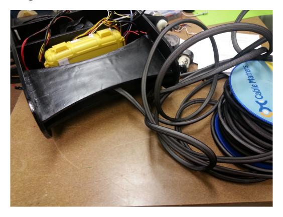
Figure 62: DIVER ROV with Tether
