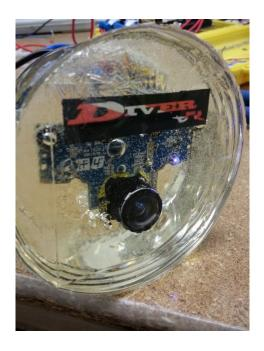
Figure 54: Camera Housing Completed
