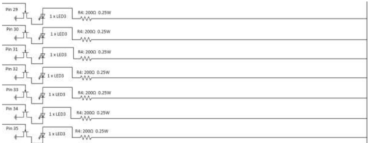
Figure 26: Circuit Diagram Channels 29-35
