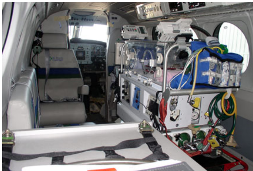
Figure 22 - Helicopter interior showing opening between patient bay and cockpit.
