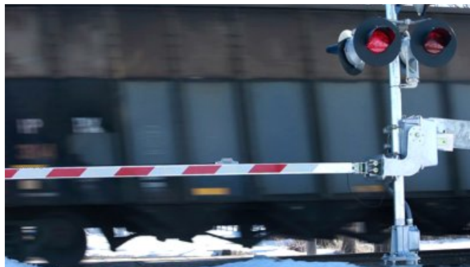
Figure 20 - Train crossing gates that may be adapted for use for road closures for helicopter landings.
