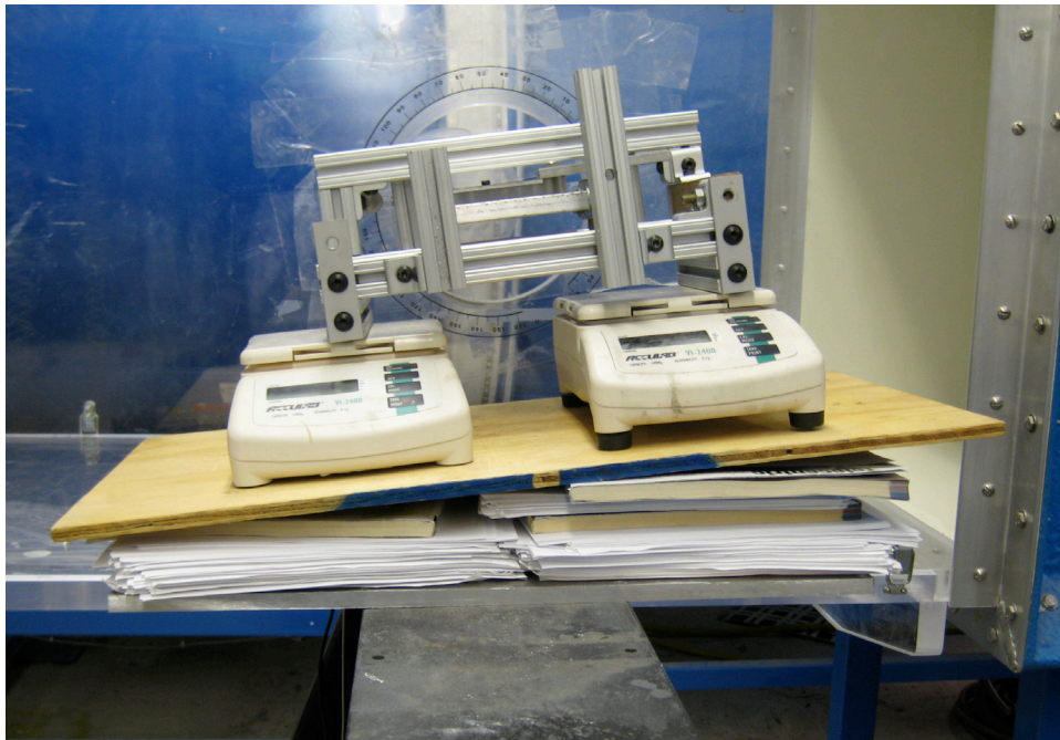
Figure 32 Equipment Setup for Normal Force Measurements
