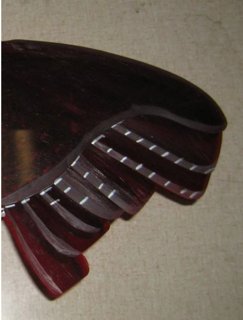
Figure 23 First Iteration Low AoA Optimized Wing
