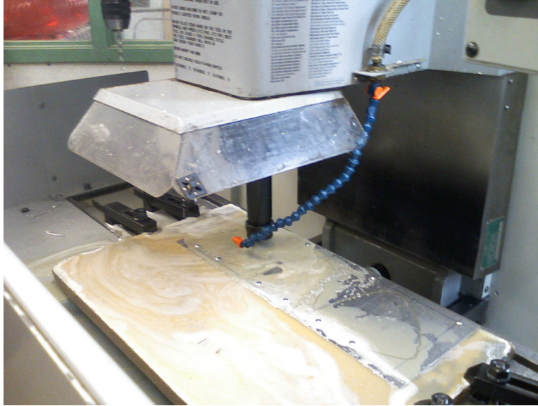
Figure 33 Machining the Wings in a CNC Mill
