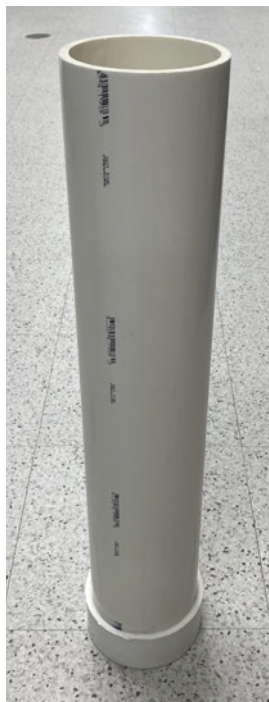
Figure C1. PVC capped pipe for acid bath
