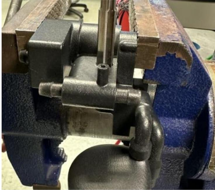
*Figure 39: Setup to ream the hole for the bypass valve in the coolant manifold.*
