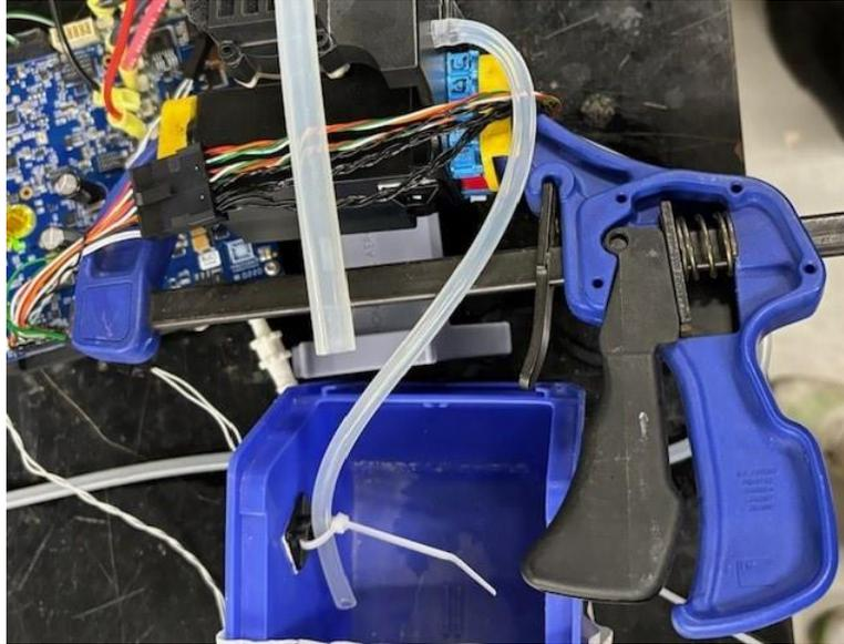
*Figure 41: Clamp applying pressure to solenoid valves.*
