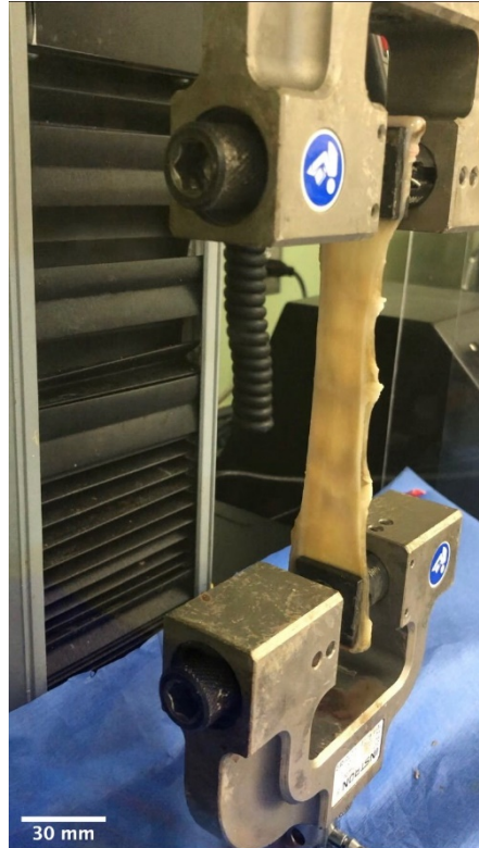
Figure 22. Tensile Test Set Up with Bovine Colon Sample on Instron 5544
