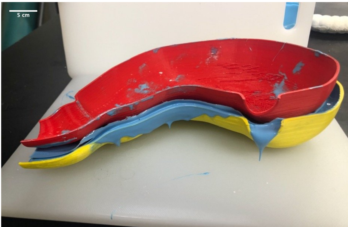
Figure 36: Stomach Compression Mold with Silicone In Between
