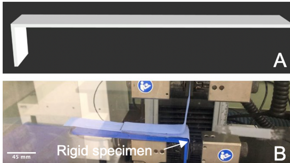
Figure 27. (A) STL file of L Shaped Rigid Specimen for Peel Testing. (B) Setup of the Peel Test with the L Shaped Rigid Specimen
