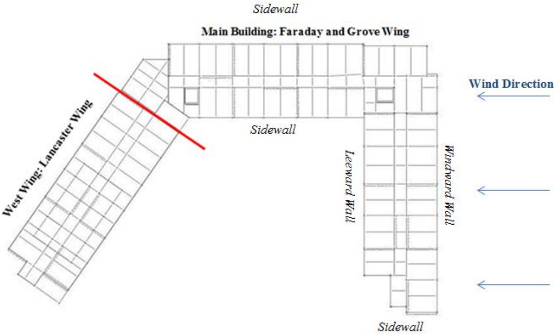
FIGURE 10: DIVISION OF BUILDING FOR WIND ANALYSIS AND DEPECTION OF WINDWARD, LEEWARD AND SIDEWALLS
