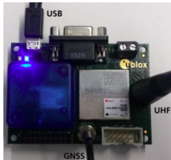
Figure 3.58: The two boards are identical. One is selected as the BASE and one as ROVER
