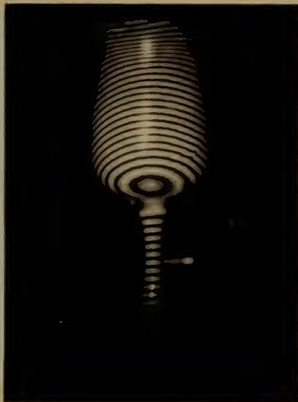
To create this double exposure hologram, one exposure was taken of the empty wine glass, another of it filled. The fringe patterns show displacement by the liquid.
