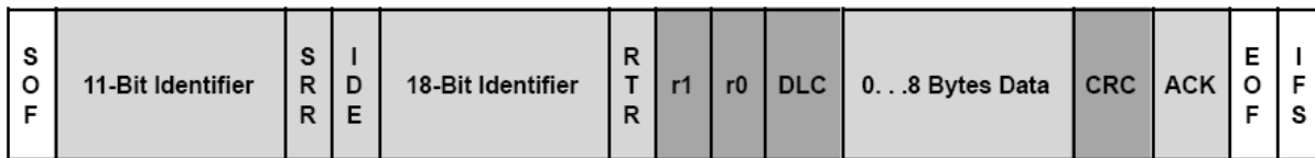
Figure 11 - Extended Frame Breakdown, Texas Instruments, Introduction to CAN
