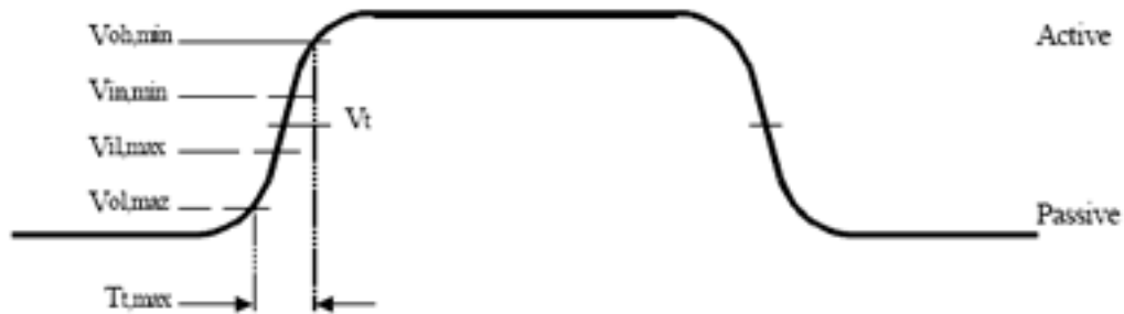
Figure 3 - SAE J1850 VPW Waveform 5
