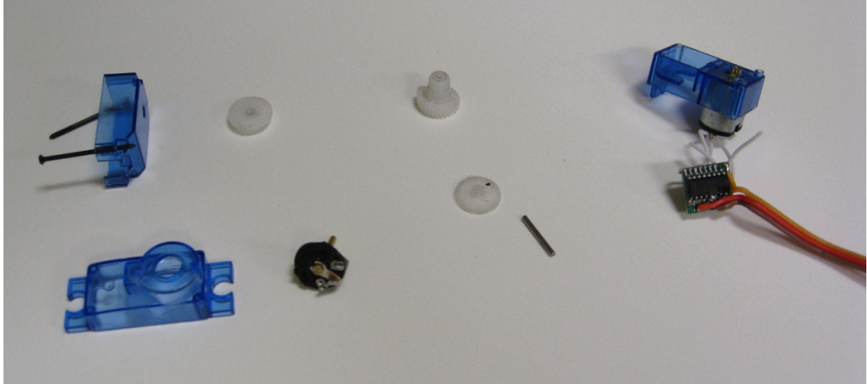
Figure 19: Parts of a Servo
