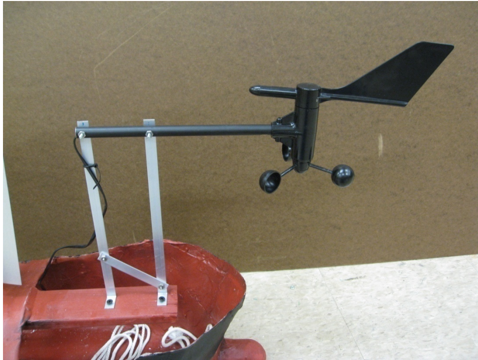
Figure 24: Annemometer and Weathervane Mounted to Hull
