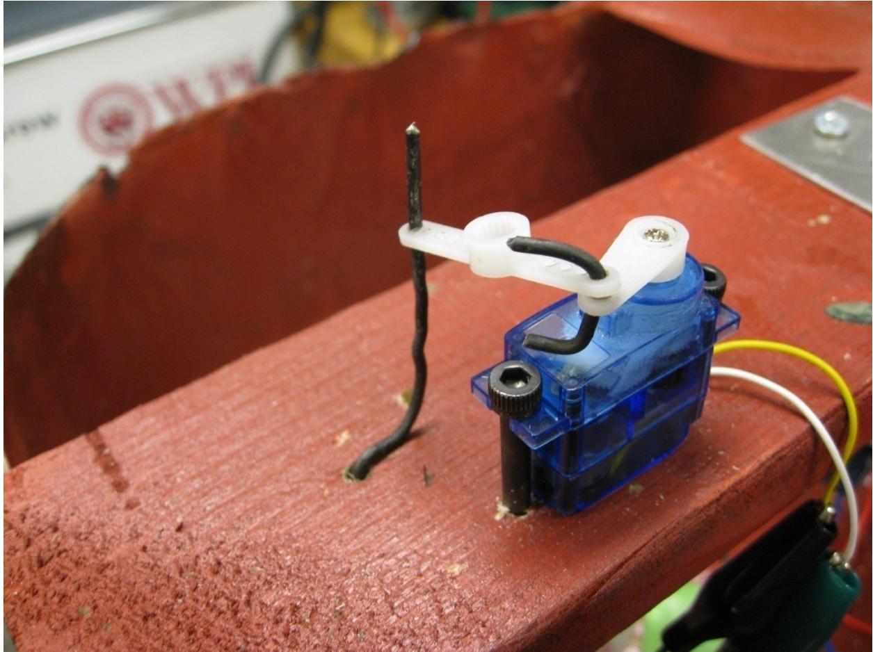
Figure 27: Four Bar Rudder Actuator
