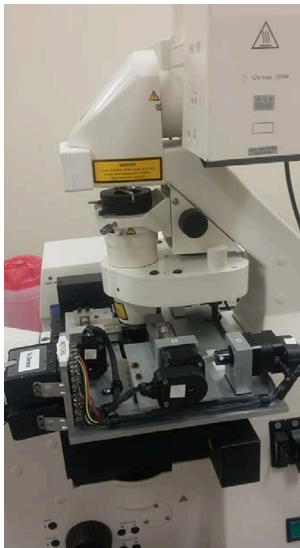
A) Panoramic view of the device used for stretching experiments.
