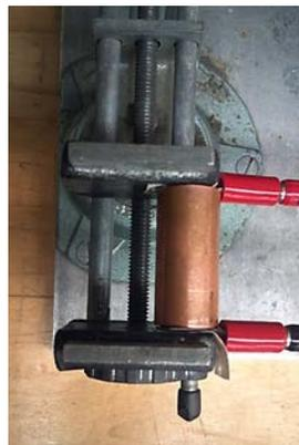
Figure 27. Four wire electrical measurement setup.
