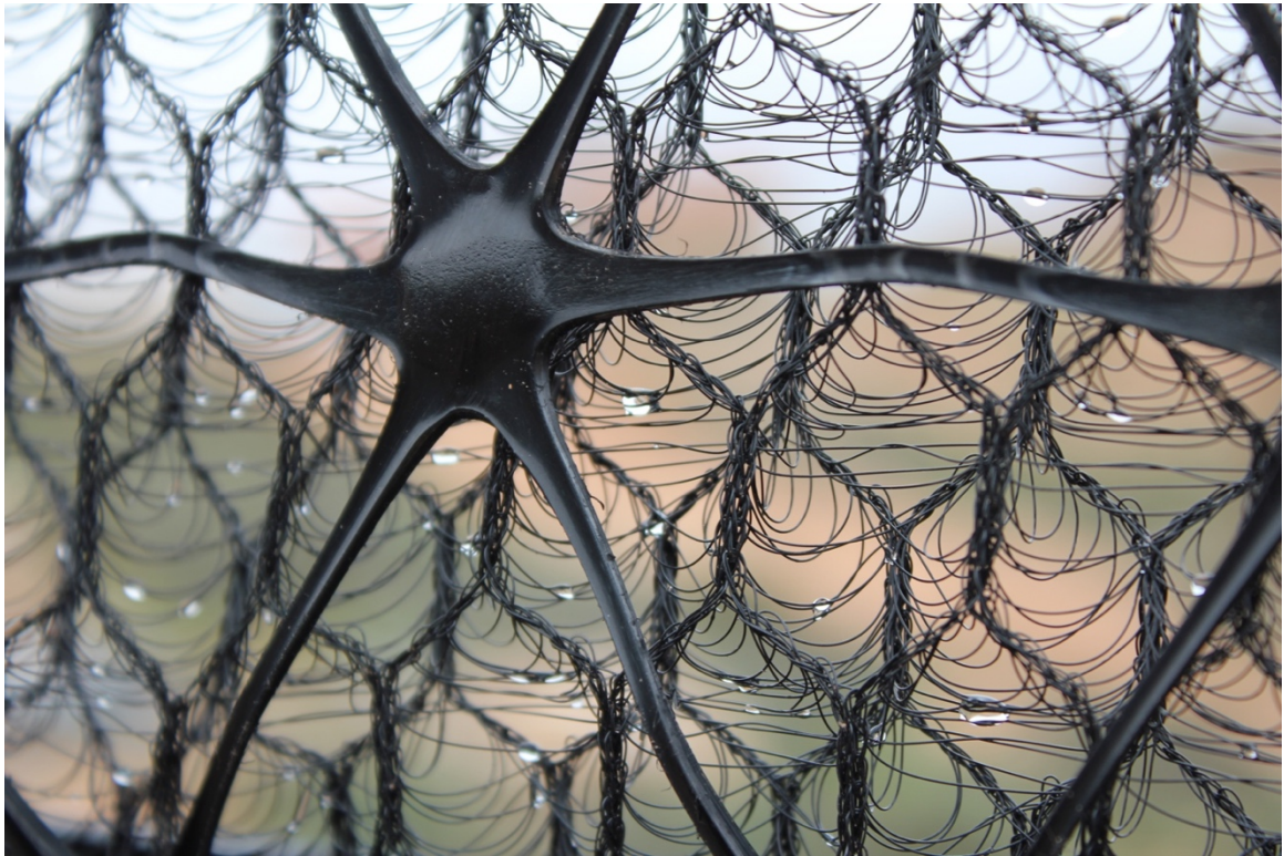
Image 4: Fog Water Condensing on Fog Net (Photo Credit: Kris Boudreau, 2015)
