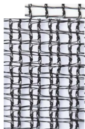
Hail net (HDPE) Net 1 dual-layer, net 2 single-layer
