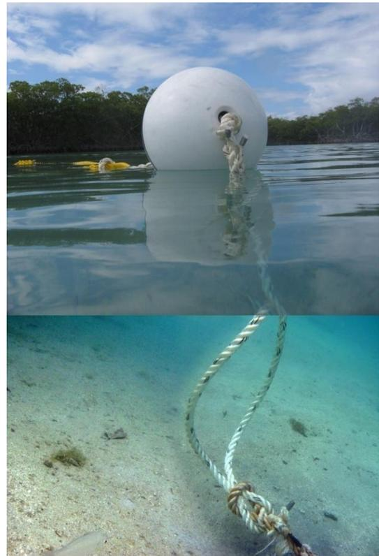
Figure 4: Mooring Buoy System
