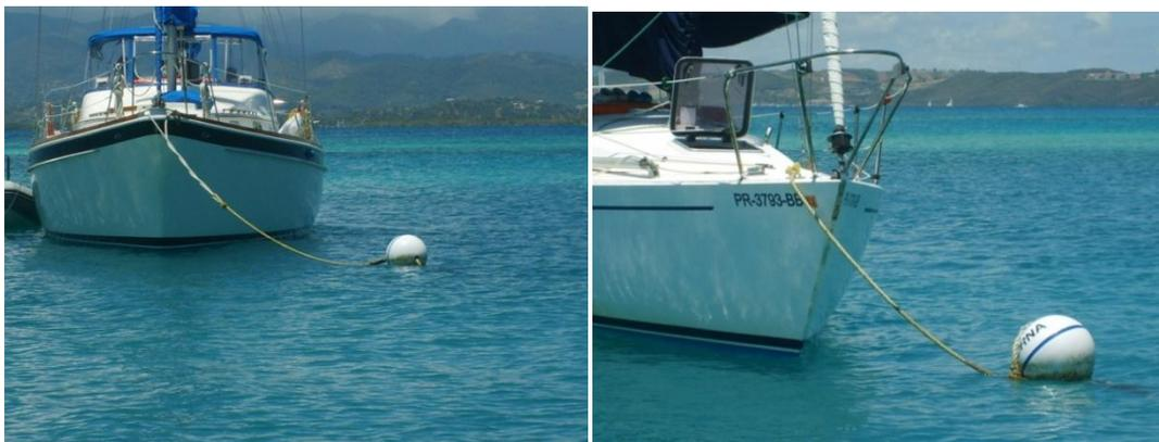
**Figure 25: Two Boats Tied to Mooring Buoys. The first picture is the correct way to moor by tying a line from the boat to the pickup line. The second picture shows the incorrect way to moor by tying the pickup line directly to the boat.**
