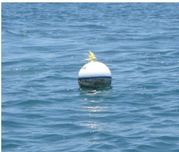
**Figure 22: A Mooring Buoy Missing Its Pickup Line**
