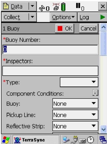
Figure 37: Buoy Data Form
