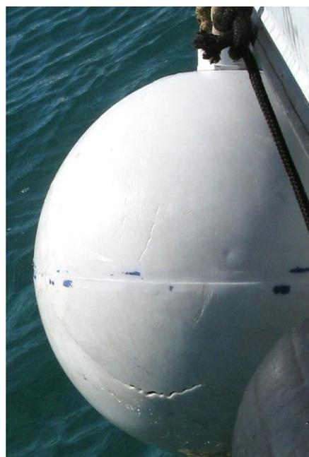
Figure 21: A Propeller Scar in the Buoy
