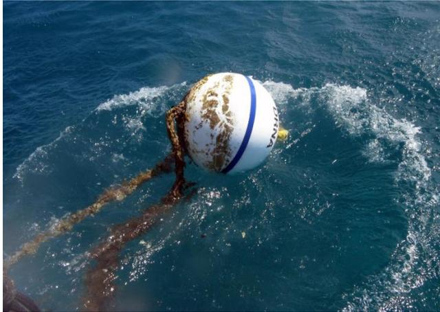
Figure 6: Growth on the Buoy and the Lines
