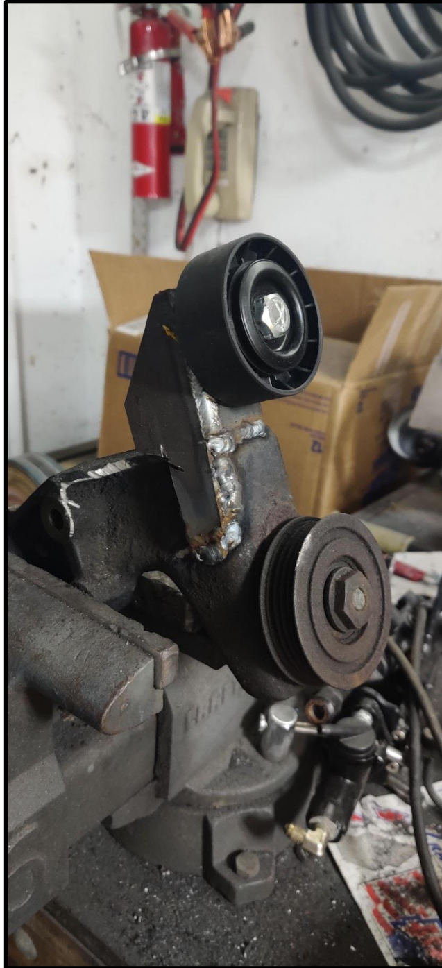
Figure 11: Belt tensioner assembly
