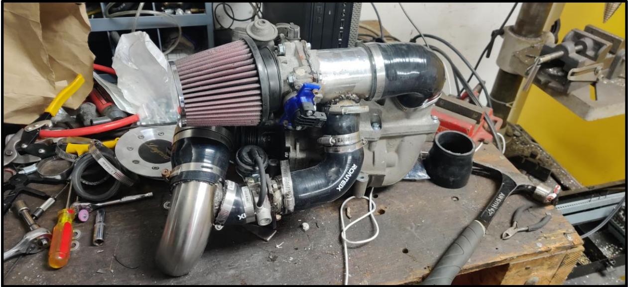
Figure 12: Supercharger and bypass valve assembly
