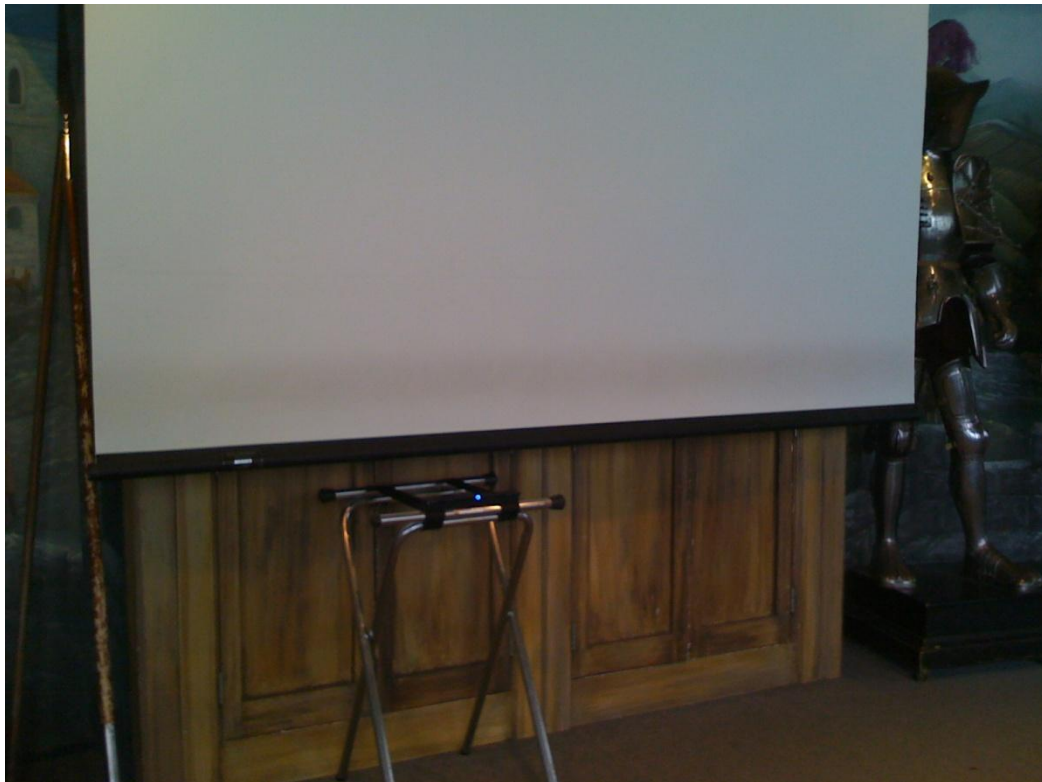
Figure 1.3.4 – A third-party sensor bar (has a single blue LED light lit) placed underneath a projector screen.
