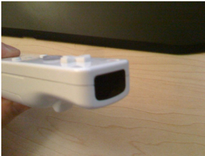
Figure 4.1.1 – The infrared sensor (black rectangle) on the Nintendo Wii Remote.
