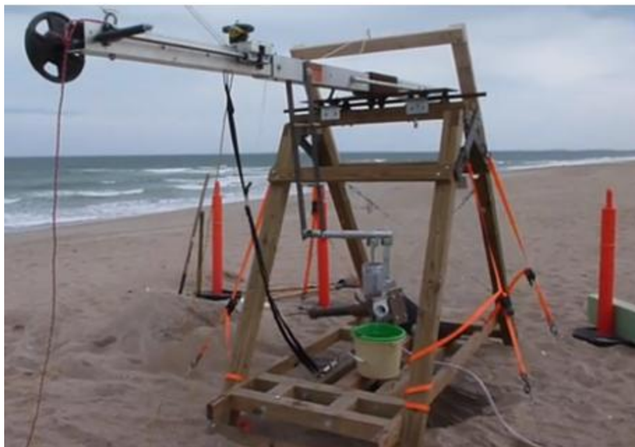
Figure 32: Snapshot of Kite-Powered Water Pump System Pumping Water
