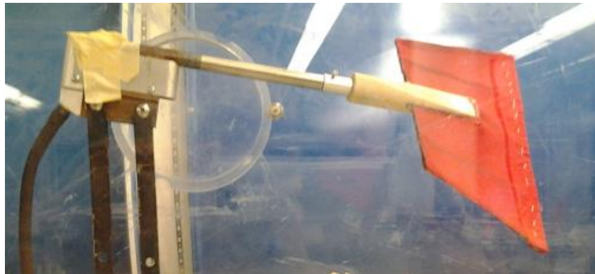
Figure 40: Kite at -10° Angle of Attack During Wind Tunnel Testing
