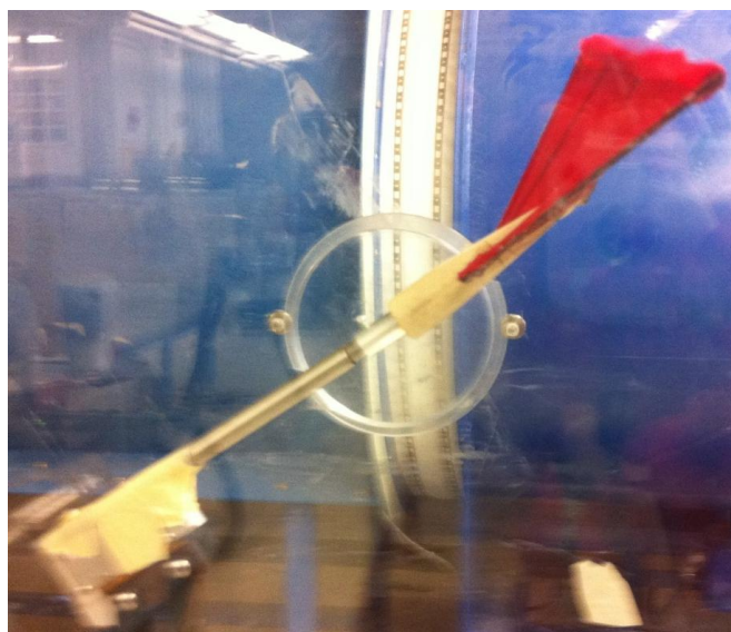
Figure 41: Kite at 30° Angle of Attack During Wind Tunnel Testing
