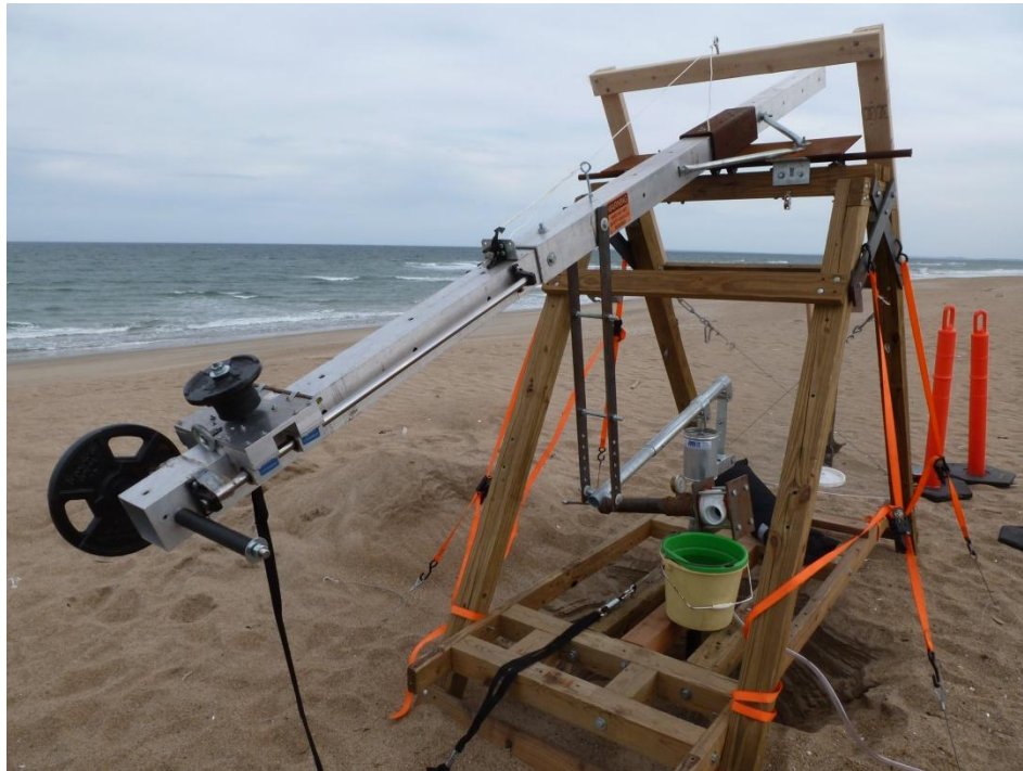
Figure 31: Kite-Powered Water Pump System with Rocking Arm Down
