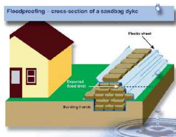
Figure 27: Residential installation of sandbag dike (New Brunswick, 1989)
