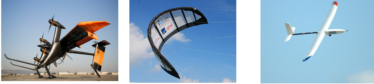
Figure 1.4: Rigid and Flexible GroundGen Airborne Kite Energy System, From [3, 4], Copyright Ampyx, Delft University of Technology
