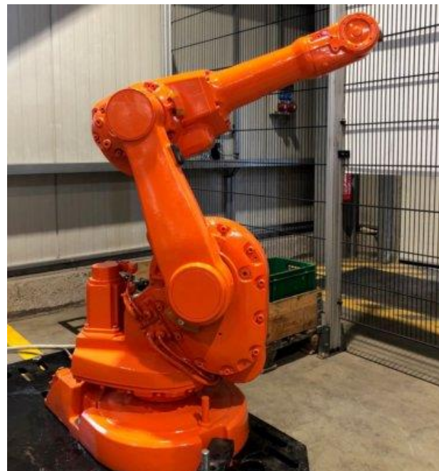
Figure 1: ABB IRB 1600 Serial Manipulator
