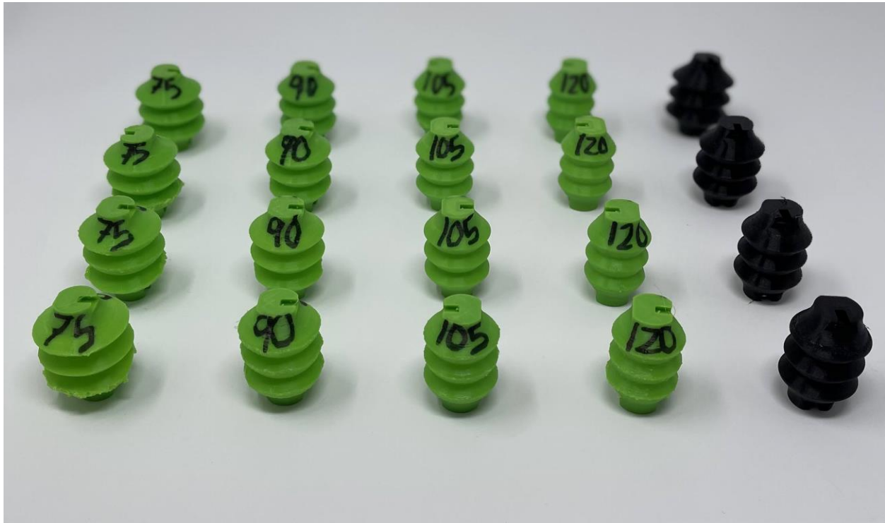
Figure 9: Factorial Experiment of Bellowed Actuator Parameters
