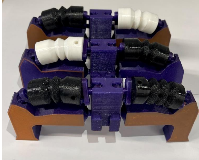
Figure 12: Constructed Bellowed Actuator Robot
