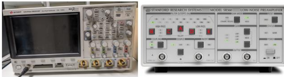
Figure 1.1: (Left) MSOX3104T mixed-signal oscilloscope with FFT capability, (Right) SR560 LNA
