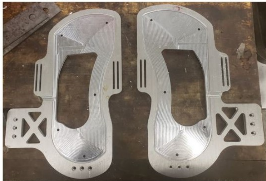
Figure 2.8: (Top) Multiple views of the Metal Footplate component, displaying each of the main features within the design. (Bottom) Both the Left and Right Footplate components flipped upside-down immediately after manufacturing. The thin cavity where the Sole-Sensor is installed is clearly visible, as are the marks made by the end-mill used to carve it out.
