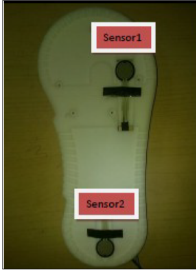
Figure 1.5: The sole of one powered DAFO device with Force Sensing Resistor sensors embedded inside. The FSRs allow the device to detect the different transition events that occur during normal walking gait [13].
