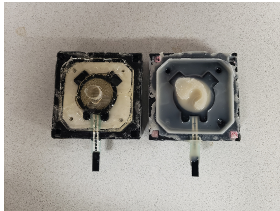
Figure 3.4: Two FSR sensors encased within two different types of Polyurethane rubber resins. (Left) Vytaflex-20 (Right) Vytaflex-30
