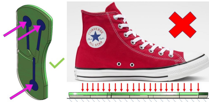
Figure 3.9: The 1st version of the Sole-Sensor did return values when forces were applied directly on the resin areas directly above the FSRs, as shown on the Left. However, stepping on the footpads directly with one's foot (Right) causes the pressure to be distributed throughout the resin medium, reducing total displacement such that no material gets pushed up against the FSRs. This results in the FSRs returning values of 0, i.e. "no load", even when a person is standing on top of the device with one leg.
