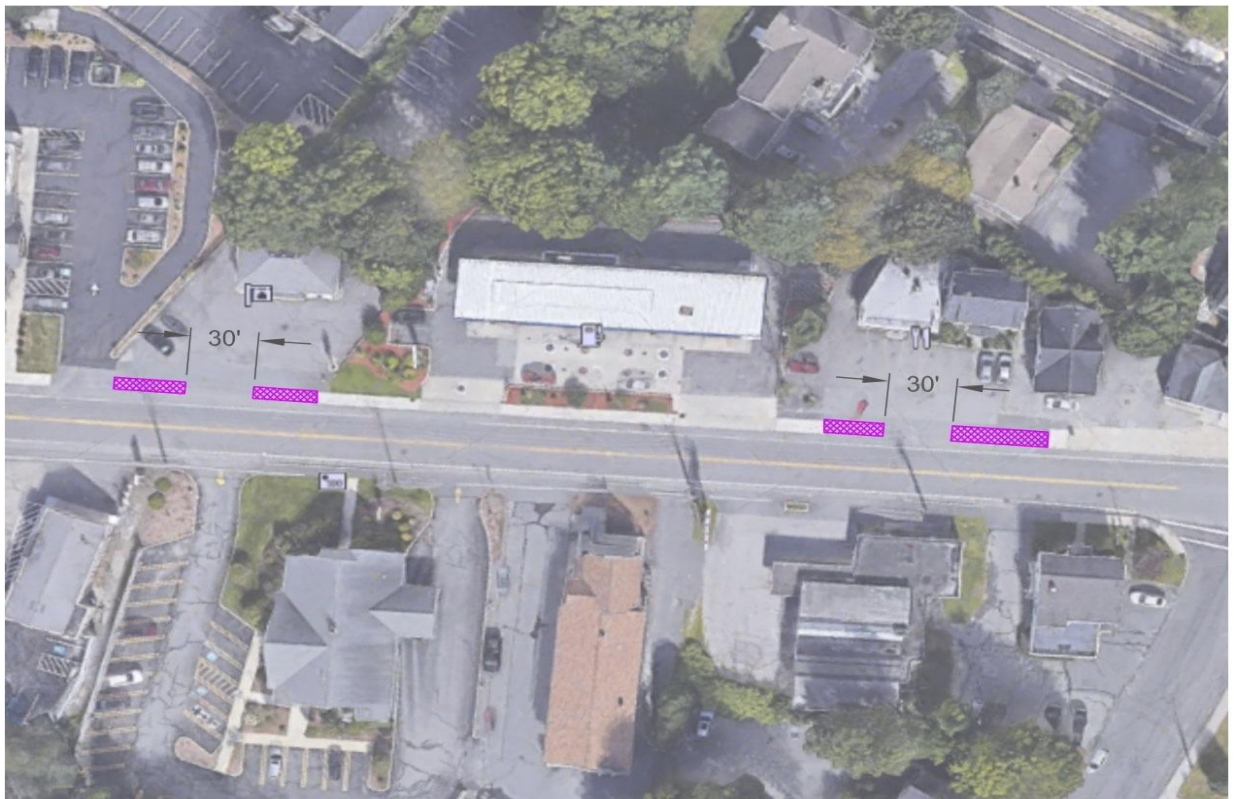
Figure 29: Placements for Continuing Sidewalks
