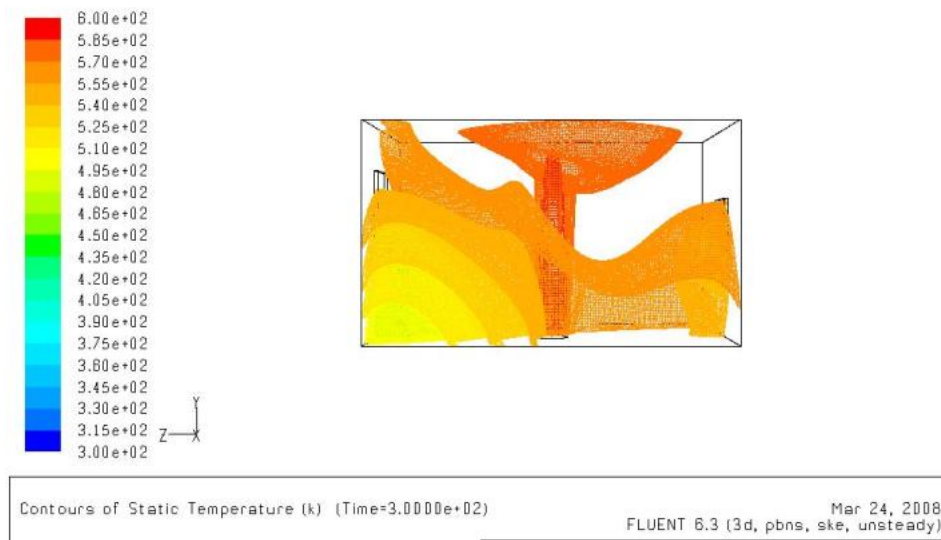
Figure 16. Temperatures in the compartment at 300s
