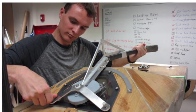
Figure 58: Hans Assembling the Movable Ballast for Testing
