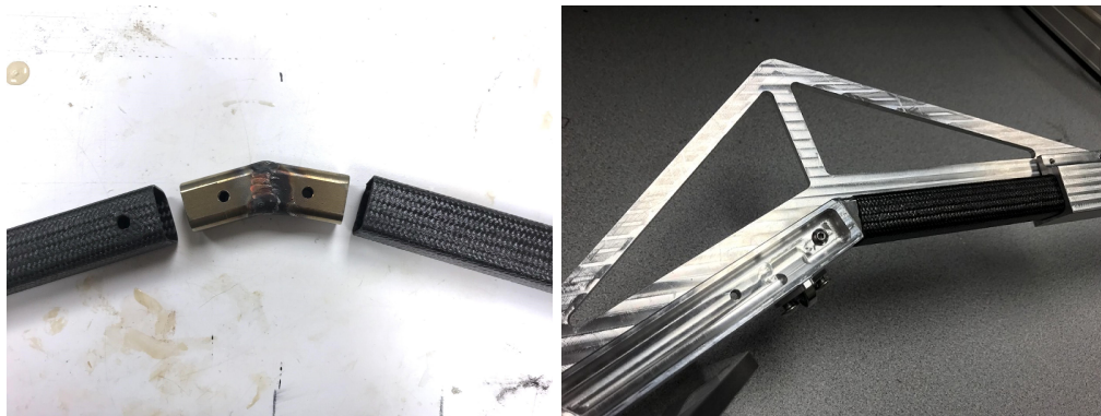
Figure 33: Original Coupler Design vs Revised
