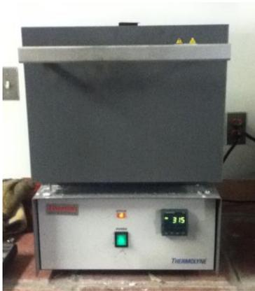
Figure 5: WPI furnace for tempering.
