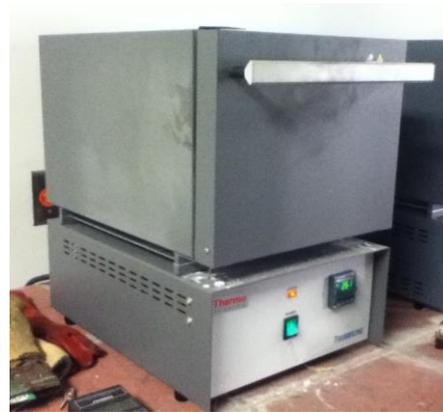
Figure 6: WPI furnace for tempering.
