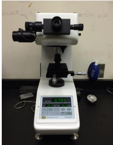
Figure 10: CM-400 AT Micro Indentation Hardness Tester.
