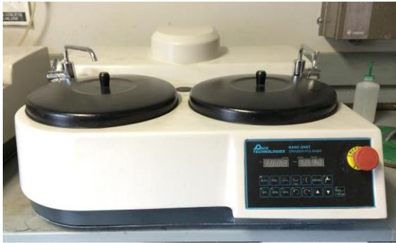
Figure 7: Pace Technologies Nano 2000T Grinder-Polisher in Washburn Laboratories.
