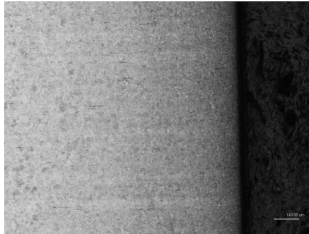
Figure 22: Photomicrograph of AISI 9310 at 5x magnification.
