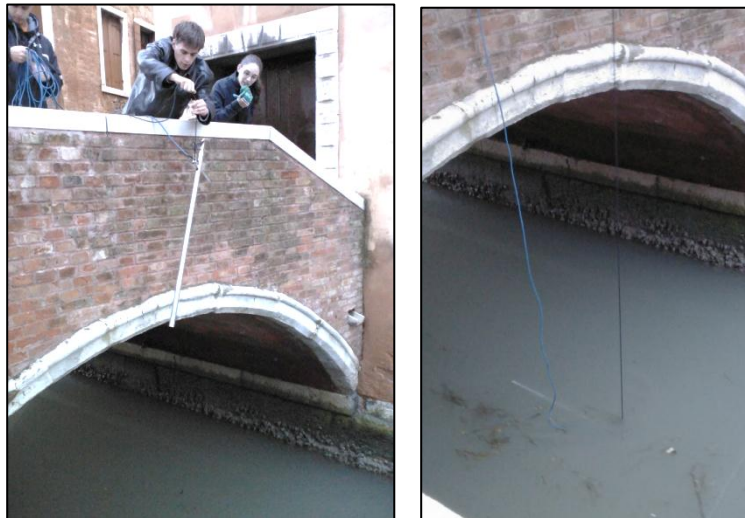
Figure 31. Left: Lowering the propeller device (with attached stabilizing pole) into a canal from a bridge. Right: The propeller device in a canal, oriented parallel to current direction
