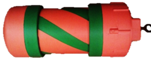
Figure 26. PVC capsule that houses the smartphone
