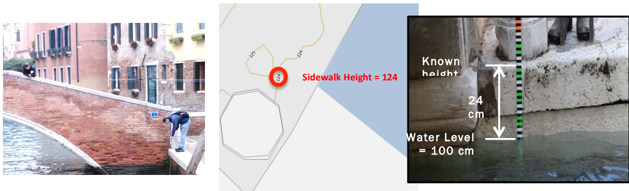
Figure 28. Left: The measuring stick is placed vertically into the canal against the sidewalk, typically near a physical landmark such as a bridge, and at least 3 photos (right) are taken for later analysis. Center: Known sidewalk height obtained from Insula. Right: Water level calculated by subtracting counted increments (24cm) from known sidewalk height
