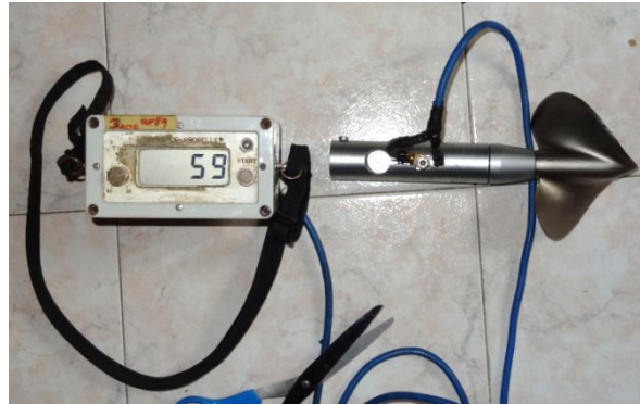
Figure 30. Head of propeller device and rotation counter from IPROS
